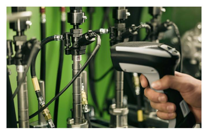
The latest exhaust emission standards and future directives increase the significance of testing common-rail injectors in modern diesel engines. Therefore, the more precise the measurement is, the more accurately the injector can be adapted.
